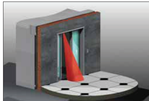
The 3D sensor projects the invisible 'cone' of infrared light out onto the landing to detect people and objects approaching the elevator.
